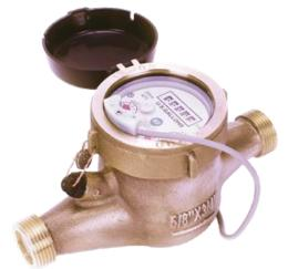
Changing the pulse rate requires no special tools and can be done in the field. This meter has a brass body and is available in 3/4", 1", 1 1/2" and 2" versions. This meter uses a two-wire reed switch. They provide a dry contact closure and do not require power.
