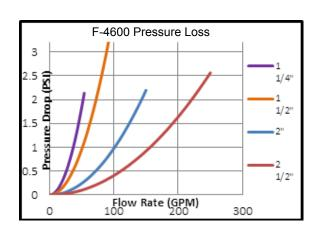
\*ONICON defines the "design" flow rate as the maximum continuous flow expected by the application under normal operating conditions. The pressure drop for the ONICON design flow rates are  $\leq 1.7$  psi.
