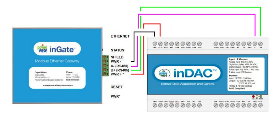
\* DC power terminals are interconnected. Do not connect to multiple power sources.
