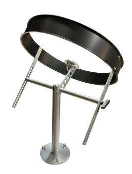
Once installed, the axis of the shadow ring must be always parallel to the polar-axis. In consequence the angle between shadow ring axis and horizontal should be equal to the latitude of the observation site.
