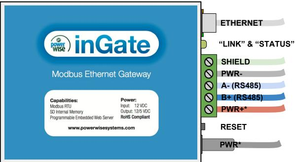
\* DC power terminals are interconnected. Do not connect to multiple power sources.
