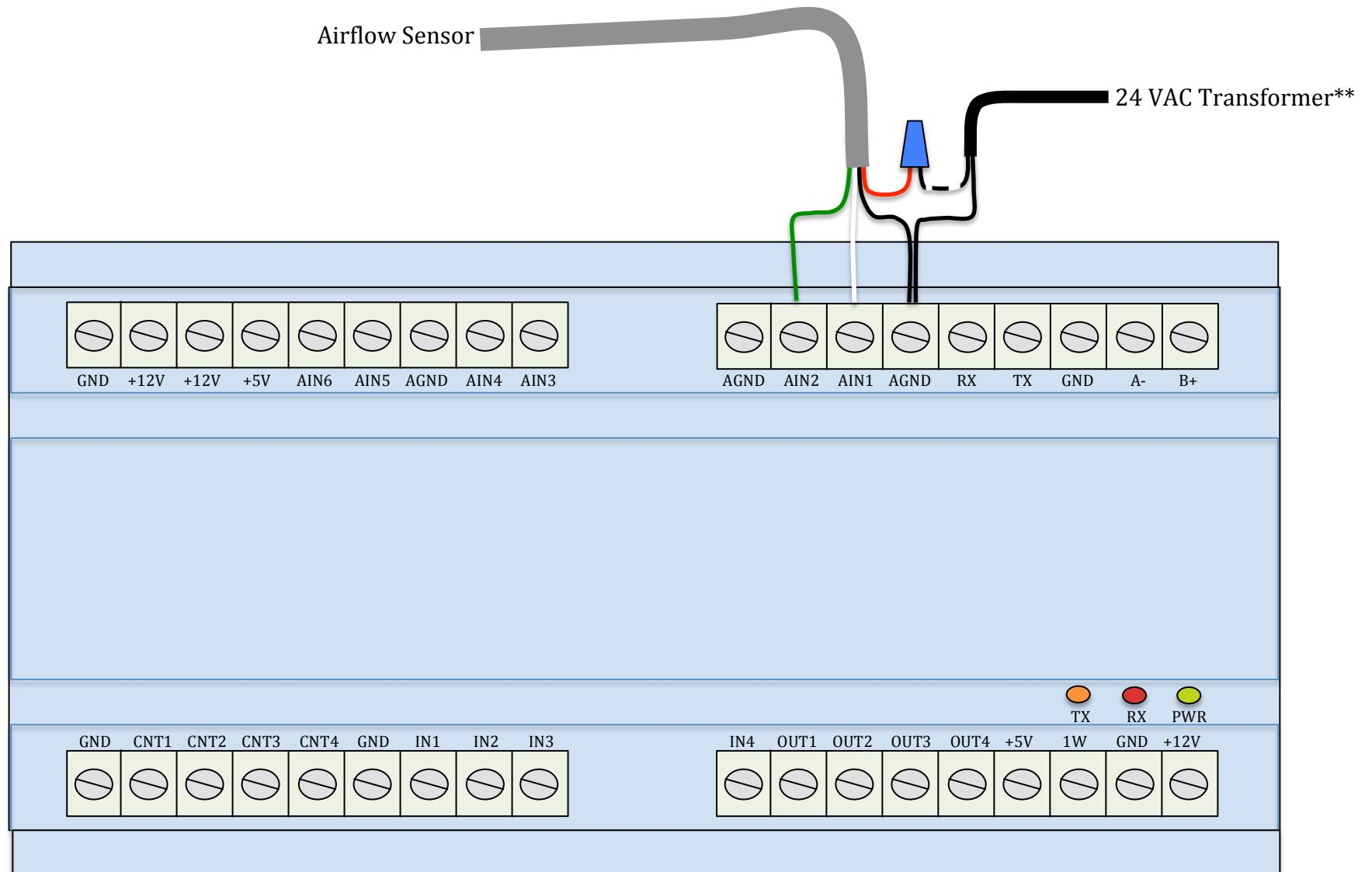
\*\* - 24VAC common must be shared with ground in order to not damage inDAC & airflow sensor.
