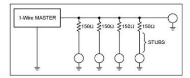
The most successful implementation of this concept uses  $150\Omega$  resistors at each point where a stub is connected to the main trunk. This value reduces the mismatch at the connection point by about 20%, and attenuates the resulting stub reflections by about 40%. However, the added resistance also degrades noise immunity by about 80%, so caution must be observed. Tests have also shown good performance using  $100\Omega$  resistor values, which do not degrade noise immunity quite as much.
