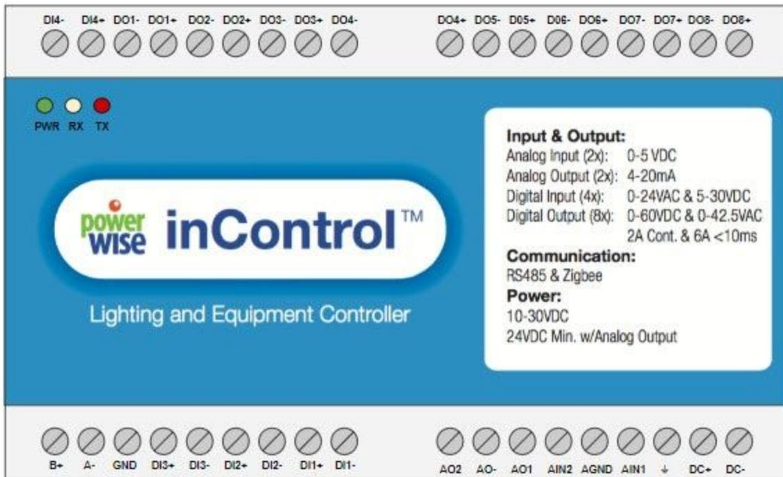
Figure 12. inControl terminal connections.
