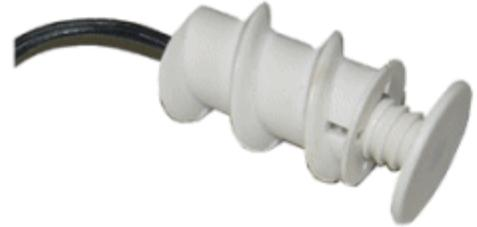
This Flush Mount temperature sensor can be screwed directly into the drywall and painted over to become almost invisible to the occupant. The 1-wire sensor element used is a DS18B20 with 12-bit resolution.
